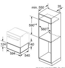
measurements in mm
