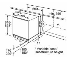
Space for electrical connection next to the appliance on the left or right-hand side. Ventilation space in the base.
