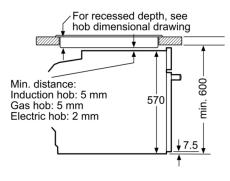
measurements in mm
