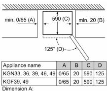
In models with vertical integrated handles, in order to open easily, a minimum distance of 65 mm is needed.
