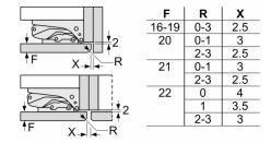
The gap dimensions recommended in the table must be adhered to in order to ensure that appliance doors do not collide with anything when they are opened, and to avoid causing damage to kitchen units.
