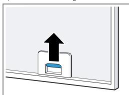
**3.** Remove the grease filters from the holders. To prevent grease from dripping, hold the grease filter horizontally.
