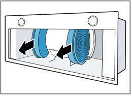
**3.** Guide the odour filter around the motor.
