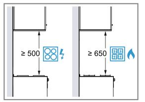
For Australia and New Zealand the minimum safety clearance above electrical cooktops must be 600 mm.
