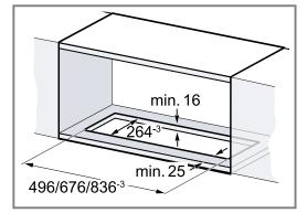
2. Make the cut-out for the exhaust air pipe either above the fitted unit or behind the fitted unit.
