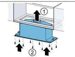
**2.** Tighten the fastening screws.
