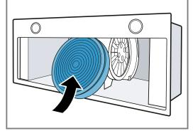
2. Guide the odour filter around the motor.
