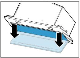
3. Undo the hinge lock and remove the filter cover.
