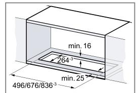
**2.** Make the cut-out for the exhaust air pipe either above the fitted unit or behind the fitted unit.
