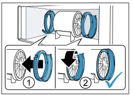
2. Slide the odour filter into the filter retainer.
