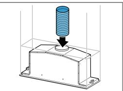
Establish the connection to the exhaust air opening.
