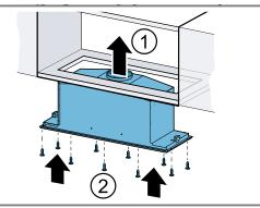
2. Tighten the fastening screws.
