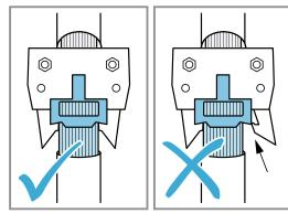
Fit the grease filters. To avoid causing damage, do not bend the grease filters.
