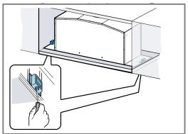
**3.** Attach the frame and screw it to the appliance from below.
