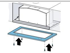
4. Secure the frame and the appliance with screws.
