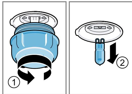
4. Insert the new halogen lamp and press it firmly into the socket.
