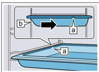
**Narrow universal pans** On the narrow universal pans, the notch **a** is in the middle. Insert the narrow universal pans with the handle **b** facing the appliance door.
