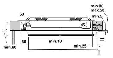
If an oven is positioned below the cooktop the barrier does not need to be fitted, but a space of 35 mm must be maintained between the underside of the cooktop and the top of the oven.
