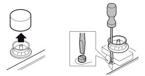
**Never remove the valve reinforcing ring.** The valve reinforcing rings guarantee the watertightness of the appliance's interior from liquids and dirt, which might otherwise prevent its correct operation.
