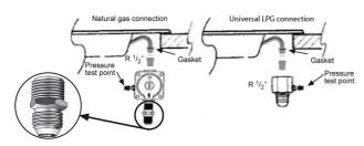
Direction of gas flow is indicated on the rear of the regulator.
