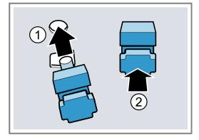
**3.** Hook the rear retainers with the hook into the top hole  $\bigcirc$  and push them into the bottom hole  $\bigcirc$ .
