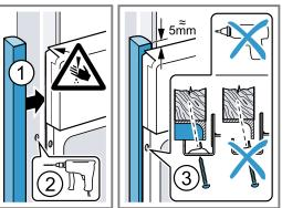
7. Refit the panels and screw them in place, first at the top and then at the bottom.
