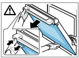
Remove the front pane and set it down on a soft, flat surface.
