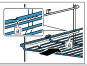
Baking tray E.g. universal pan or baking tray Slide the tray in with the sloping edge **b** towards the appliance door.
