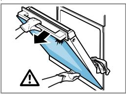
If you are unable to release the front pane, take hold of the top edge of the front pane and pull it in the direction of the arrow.
