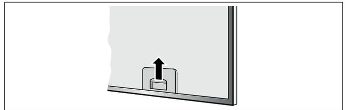
1. Open the lock on the metal grease filters and remove the filters from the retainer.
