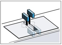
6. Insert the grease filter.
