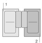
**Note:** With the flexible cooking zone, the ShortBoost function can be activated even if it is used as the only cooking zone.
